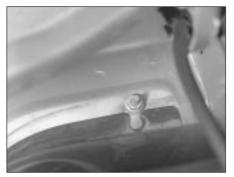
16.6b ... then disengage the right-hand half of the panel from under its single retaining nut (left-hand shown)
